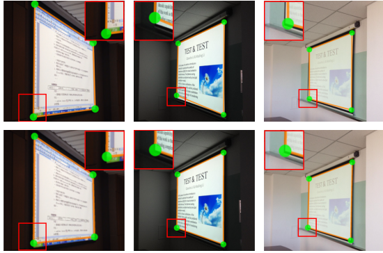
Fig. 6. Comparison of the quadrangle detection results. From left to right: pic 0 , pic 1 and pic 2 . From top to bottom: CaptureBoard and the proposed method.
